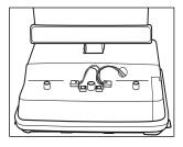
Remove lamp housing by removing two (2) screws in the the top of the lamp housing. Pull burned out bulb from holder and replace with new bulb. Use only Oreck replacement parts. Reassemble lamp housing by replacing two screws in the top of the lamp housing. WARNING: Unplug cord from electrical outlet before servicing.
